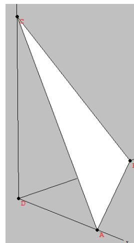
Another 3-d analogy of the Pythagorean Theorem is de Gua's Theorem. If a tetrahedron has all right triangles for the three faces meeting at one vertex (D in the image at right), de Gua showed that if the areas of the three right angled triangles are A, B, and C, and the triangle on the base has area D, then  $A^2 + B^2 + C^2 = D^2$ . Notice that
